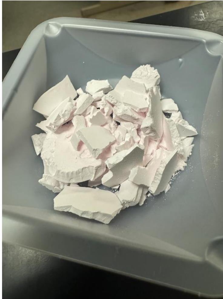
*Figure 1. Battery grade crystallized  $MnSO_4$  prepared by KCA from Berenguela composite sample RD4LOWA.*
